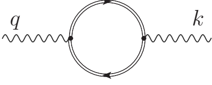
Fig. 1. Feynman diagram describing the leading-order contribution to the photon polarization operator. The amplitude of the process is proportional to the fine-structure constant \alpha and exactly takes into account the interaction with the classical external background (double lines represent the dressed Green's functions)
