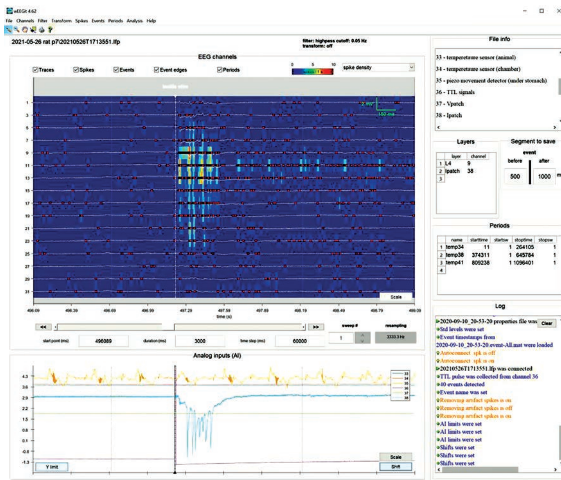
Fig. 1. WEEGIT interface view 1, using spike density as background. The main panel (EEG channels) displays amplifier channels extracted from the electrophysiological record. The additional panel (Analog inputs (AI)) displays data from other sensors (e.g., telemetry sensors) synchronized with electrophysiological data. General information panel (File info) is intended for downloading (in *.txt format) and/or creating and editing text information about the current record. The panel of morphological labels (Layers) is used for marking the correspondence of channels to morphological structures. The segment saving panel (Segment to save) contains editable time values defining intervals before and after each event (in milliseconds) that will be used to save data segments around the event timestamp. The period information panel (Periods) is used to enter/edit time period information if the user needs to mark the time period during which the experiment conditions were changed/intact. The action overview panel (Log) displays non-editable information about ongoing user actions.
