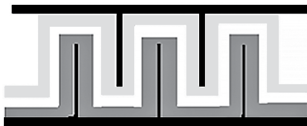
Fig. 2. 3D design with interdigital arrays of electrodes.
