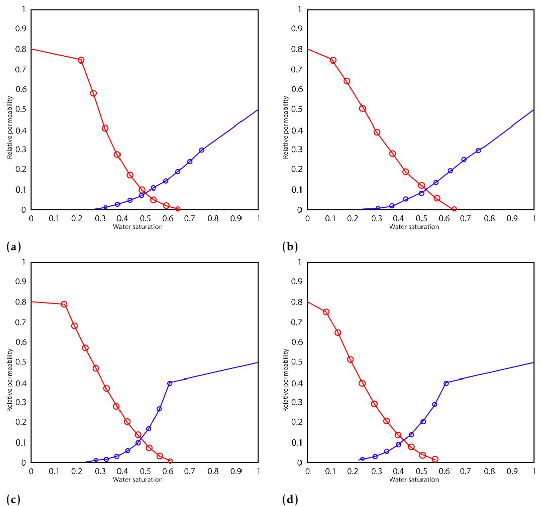
**Figure 13.** Relative permeability of the layers of Nizovsky deposit.
