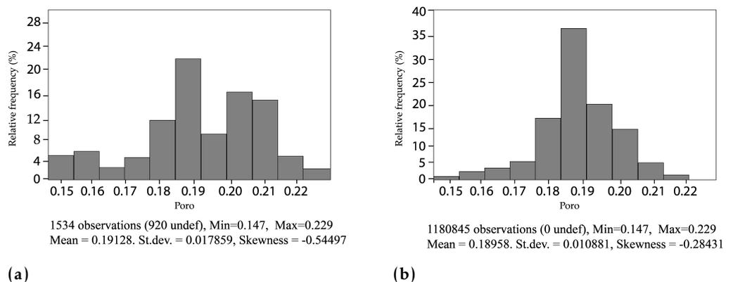
**Figure 6.** Porosity distribution of B-2 formation in wells (a) and in the formation as a whole (b).
