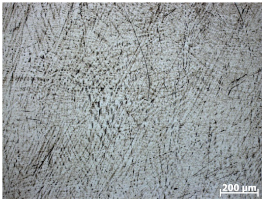
Fig. 2. Microstructure of the samples obtained using WAAM technology
