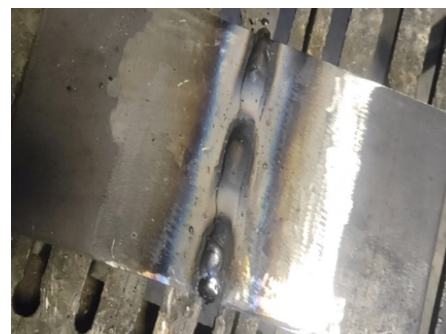
Fig. 5. Appearance of the welded seam after filling with TMU-21U electrodes CJSC “Elektrodneyi zavod” St. Petersburg:
