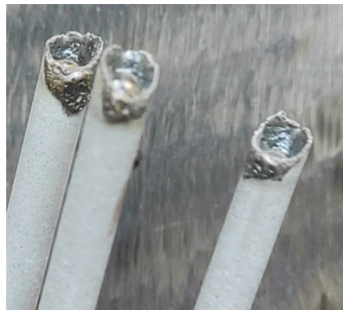
Fig. 4. Formation of the fingernail after welding with TMU-21U electrodes CJSC “Elektrodneyi zavod” St. Petersburg
