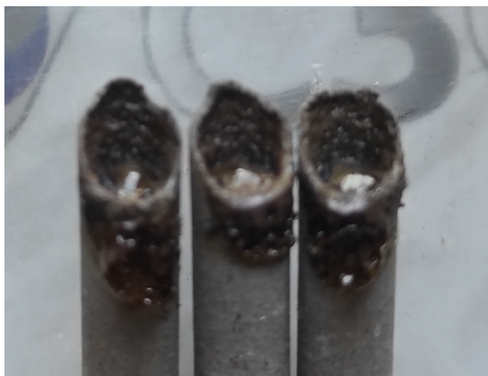
Fig. 2. Formation of a fingernail after welding on TMU-21U electrodes produced by "Sudislavsky Welding Materials Plant", LLC
