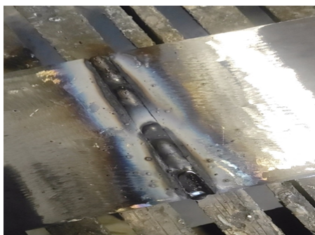
Fig. 5. Appearance of the welded seam after filling with TMU-21U electrodes CJSC “Elektrodneyi zavod” St. Petersburg:
