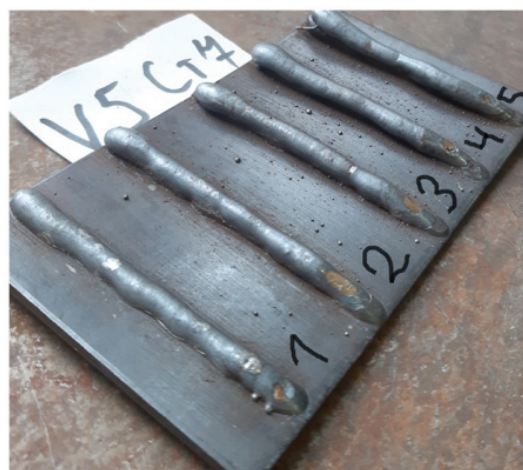
Fig. 1. Schematic diagram of the bead surfacing process (a) and a plate with surfaced beads (b)
