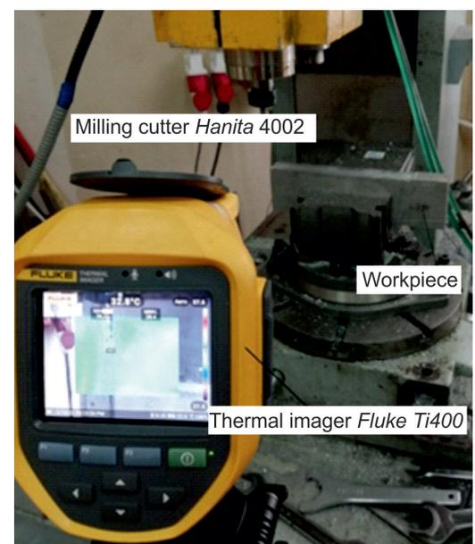
Fig. 8. Experimental system for temperature measurement
