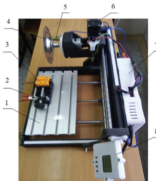
To control the electrochemical processes during the investigation, the test bench was additionally fitted with the proprietary current polarity control board and relay block, which were coordinated with the existing step motor control board of the machine. Such configured device was housed inside the integrated control unit casing made by additive manufacturing, see in fig. 4.
