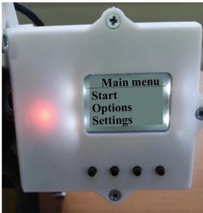
Fig. 7. Data display block for interactive operation
