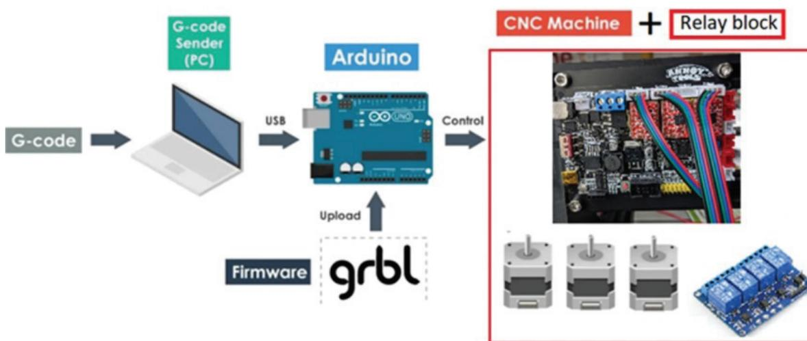
Fig. 5. Joint control circuit of machine stepper motors and relay unit
