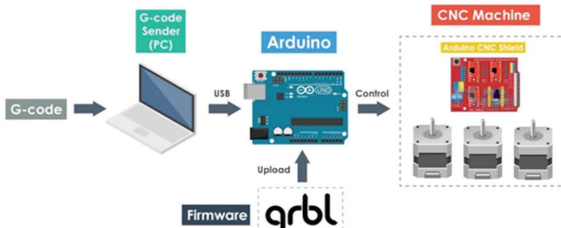
Fig. 2. CNC machine control circuit using *Arduino*
