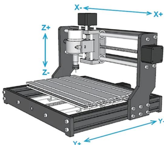
Fig. 1. Three-axis *CNC* machine
