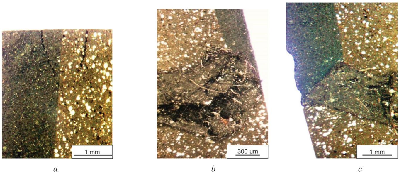
Fig. 3. Cross-section of hone teeth with surface integrity failures
