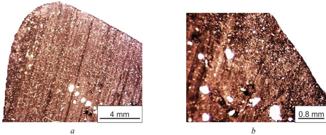
Fig. 9. Cross sections of a hone tooth using green silicon carbide powder as an abrasive material:
