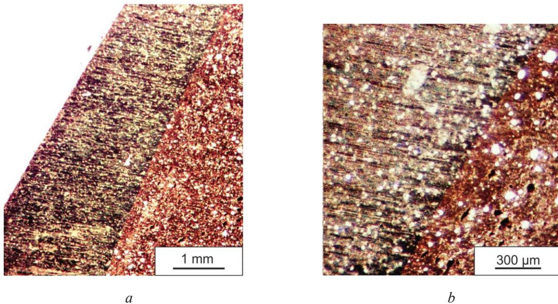
Fig. 2. Cross section of a hone tooth at magnification of 15× (a) and 50× (b)
