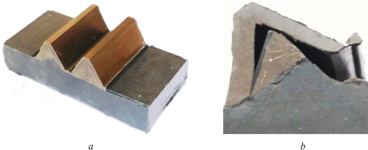
Fig. 7. Two-tooth fragment of a hone after vulcanization (*a*) and a view of the end part of a hone tooth with prevulcanized abrasive layer (*b*)
