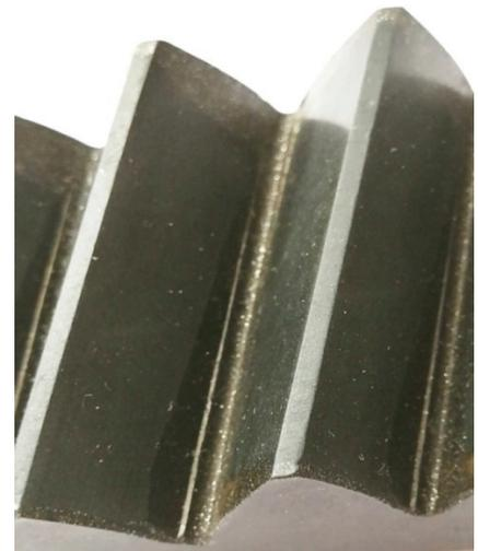
Fig. 1. Fragment of the working surface of the hone teeth
