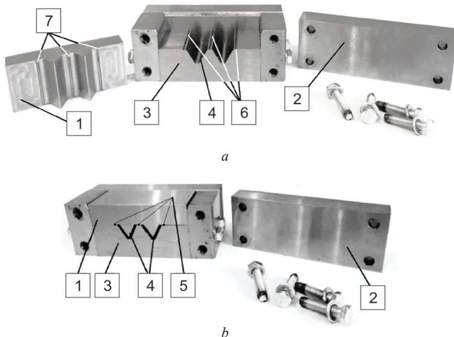
Fig. 6. A mold for forming a diamond-bearing layer (*a*) and hone teeth (*b*)
