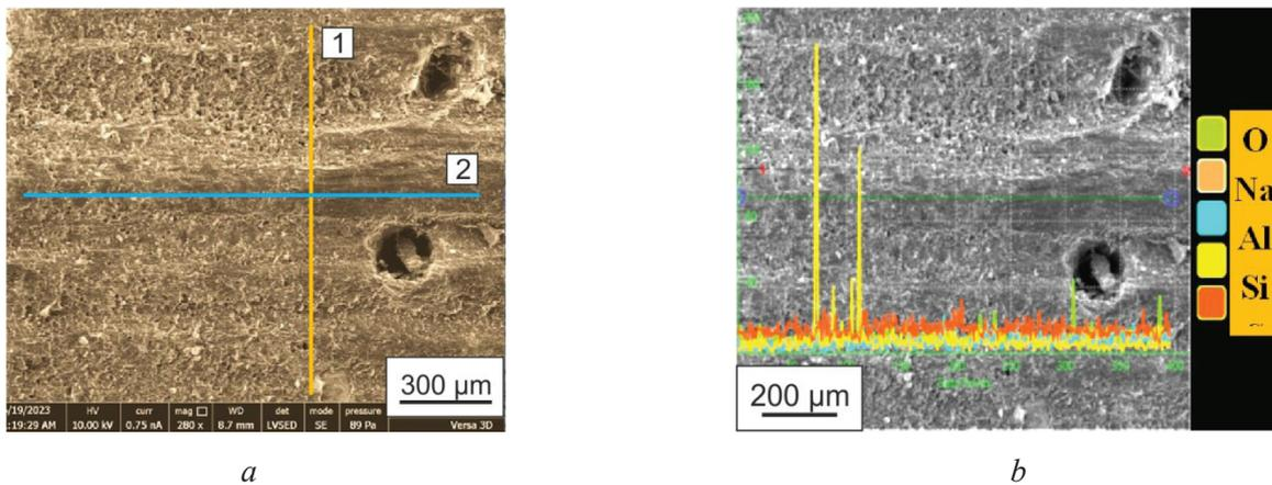
Fig. 10. Morphology and chemical composition at the interface between the abrasive layer and the gear material
