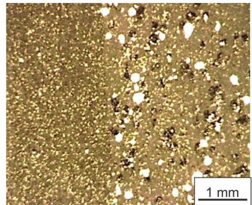
Fig. 8. Interface between the abrasive layer and the annular gear material
