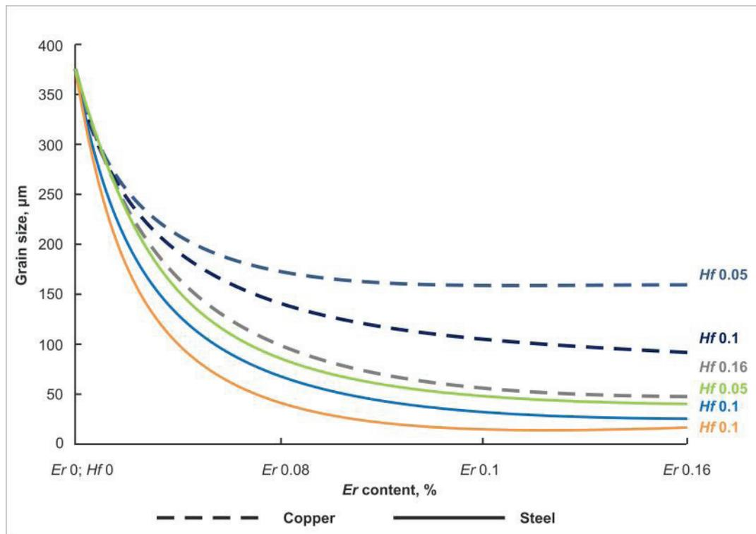
Fig. 3. Dependence of grain size on the amount of alloying components (on specimens cast into a steel and copper chill molds)
