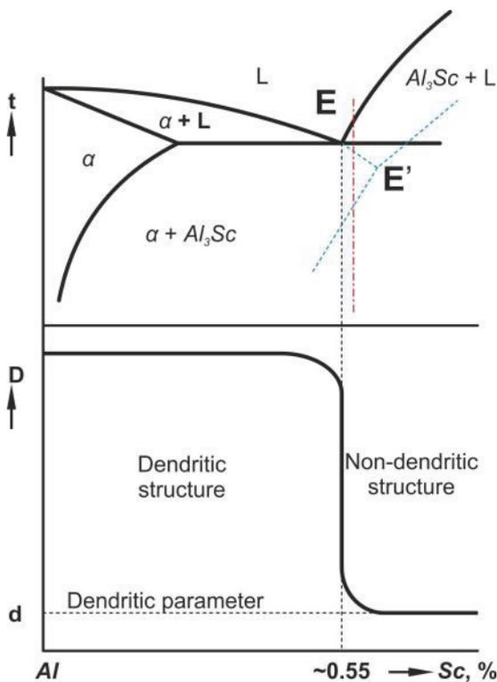
Fig. 4. Aluminum-scandium phase diagram [32]
