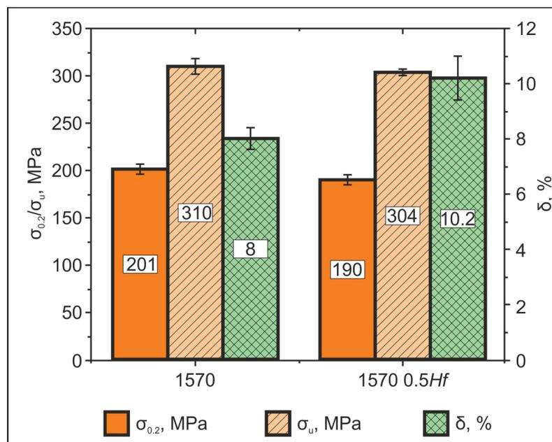
Fig. 3. Mechanical properties of studied as-cast alloys after homogenization annealing at 440°C – 4 hours
