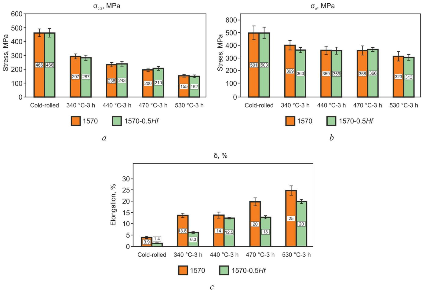
Fig. 5. Mechanical properties of 1570 and 1570–0.5Hf sheets:
