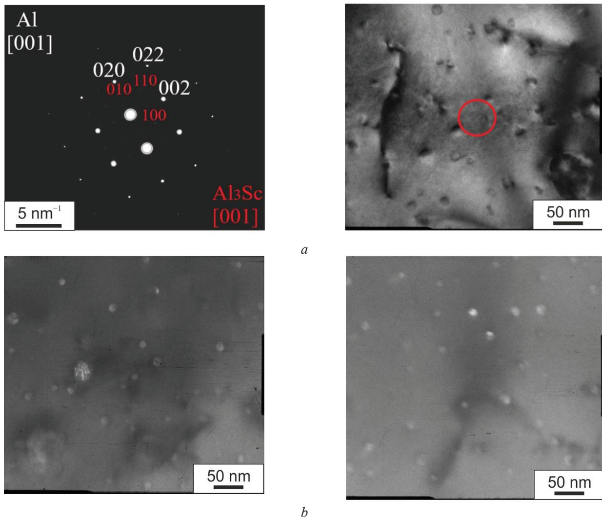
Fig. 2. Fine structure of the cast billet made of alloy 1570 0.5Hf after its homogenization annealing at 440 °C for 4 hours:
