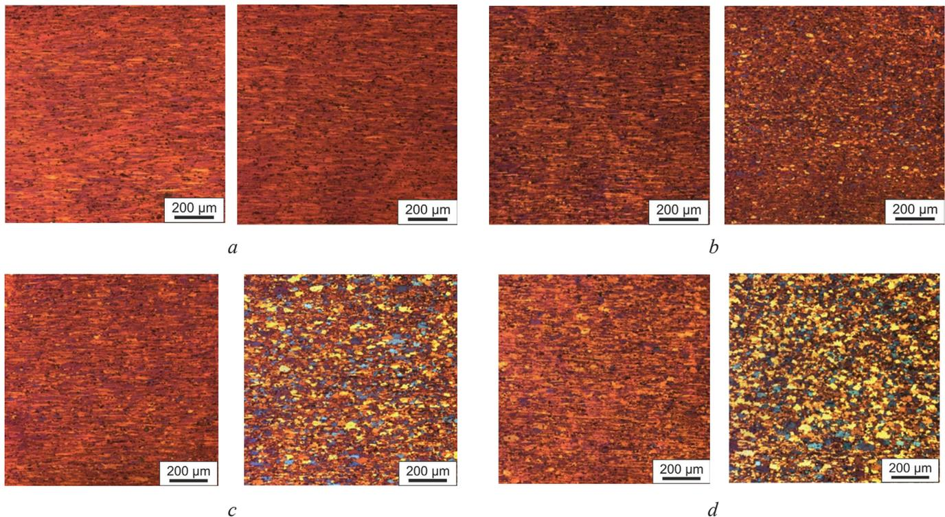
Fig. 4. Microstructure of sheets after cold rolling with 90 % deformation and subsequent annealing of alloys 1570 (left) and 1570-0.5Hf (right):
