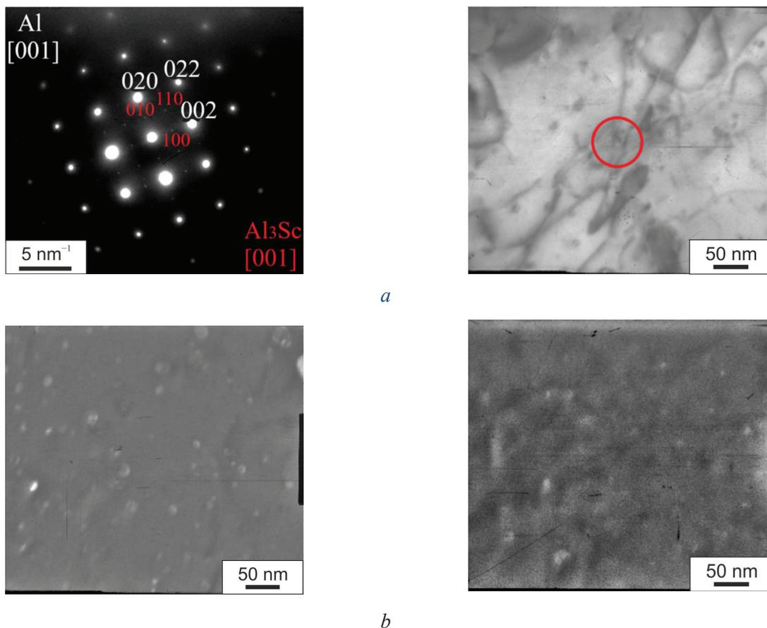
Fig. 1. Fine structure of a cast billet made of 1570 alloy after its homogenization annealing at 440 °C for 4 hours:
