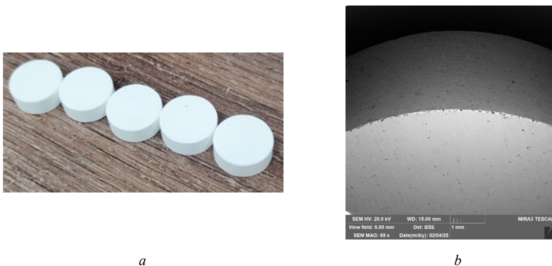
Fig. 1. Ceramic inserts (a) and electron microscopy of the cutting edge (b) in the initial state
