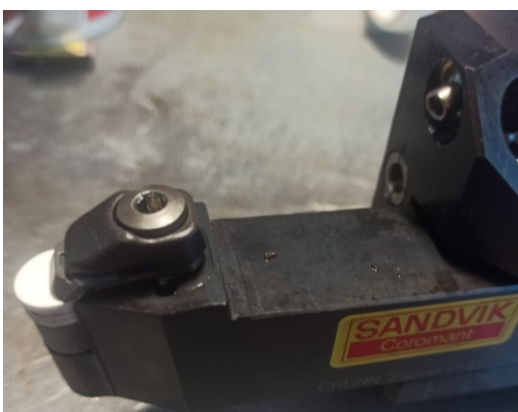
Fig. 2. Mandrel with a ceramic insert attached
