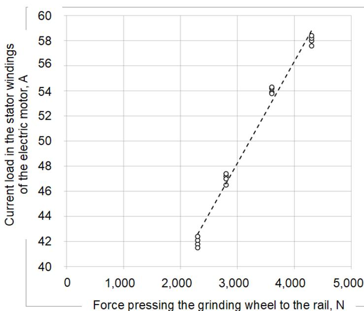
Fig. 11. Dependence of current load change in the stator windings of the electric motor on the force of pressing the grinding wheel to rail
