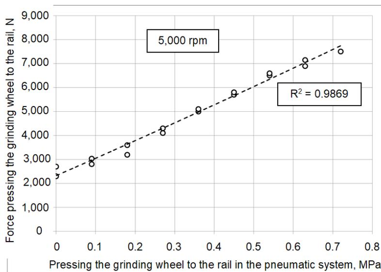
Fig. 10. Dependence of the pressing force of grinding wheel to rail on pressure in the pneumatic pressing system
