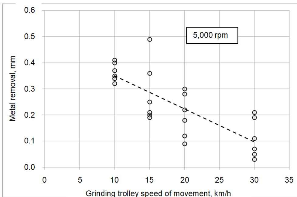
Fig. 13. Dependence of metal removal on grinding modes
