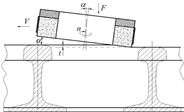
Fig. 3. Schematic representation of interaction of an abrasive tool with a rail during high-speed grinding
