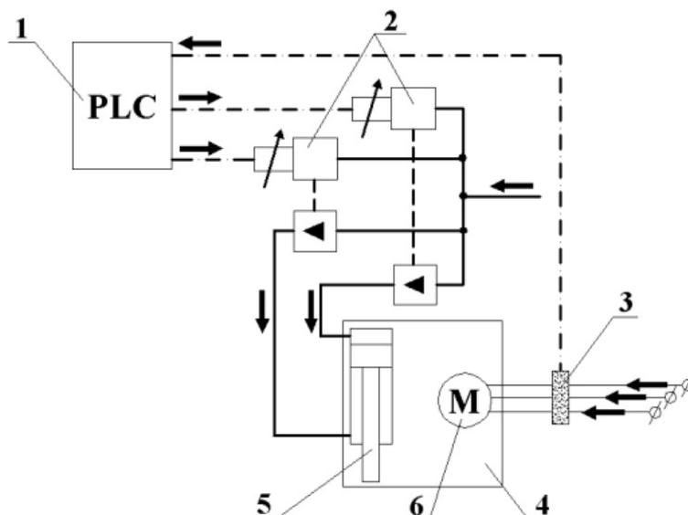
Fig. 5. The pressing force of grinding wheel common control circuit:
