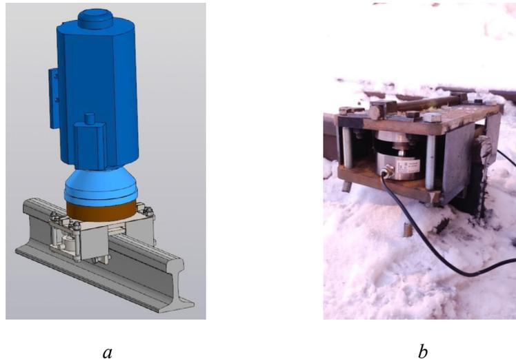
Fig. 9. Device for calibrating the pressing force of grinding wheel to rail:
