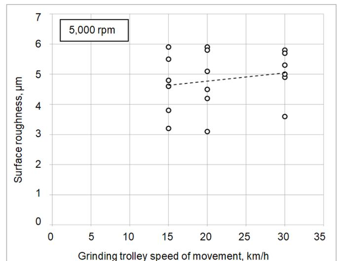
Fig. 15. Dependence of roughness of the machined surface on grinding modes
