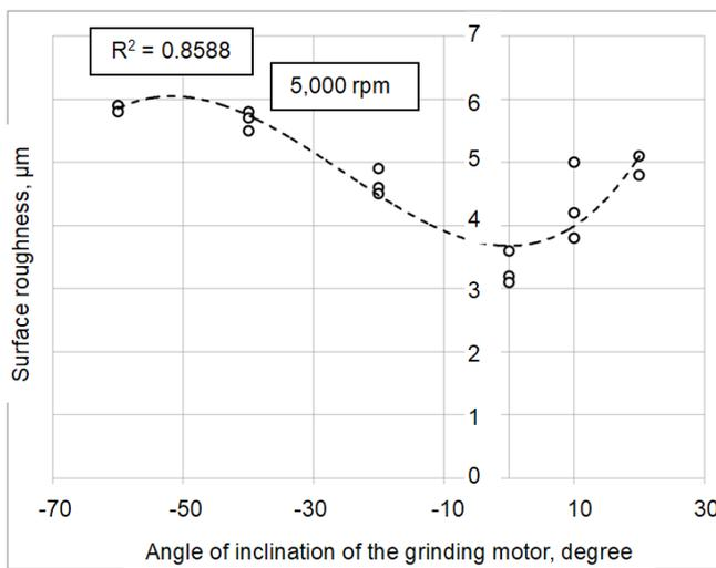
Fig. 14. Surface roughness at the angles of inclination of grinding motor
