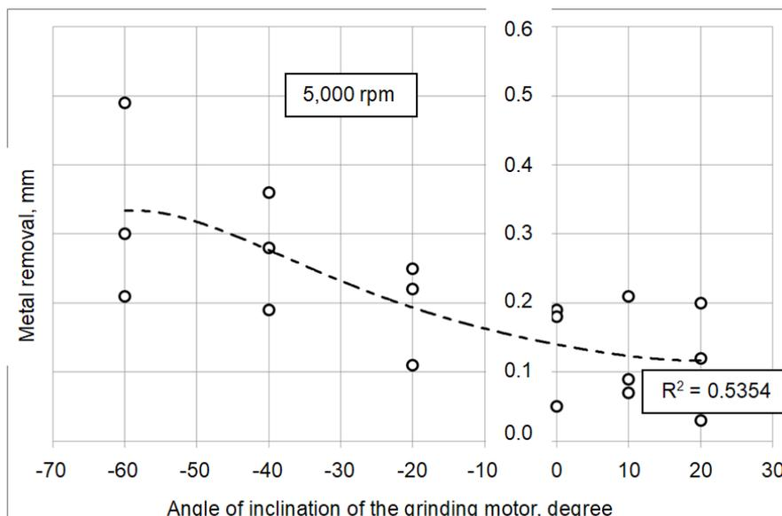
Fig. 12. Removal of metal at the angles of inclination of grinding motor
