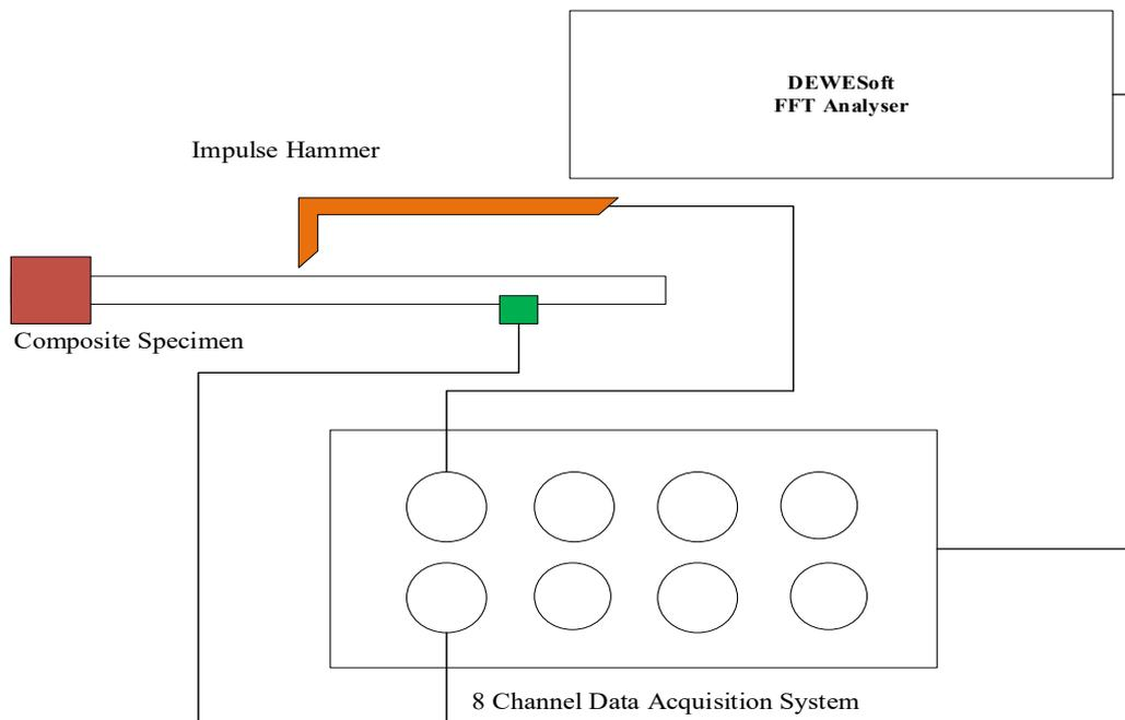
Fig. 4. Freevibration setup
