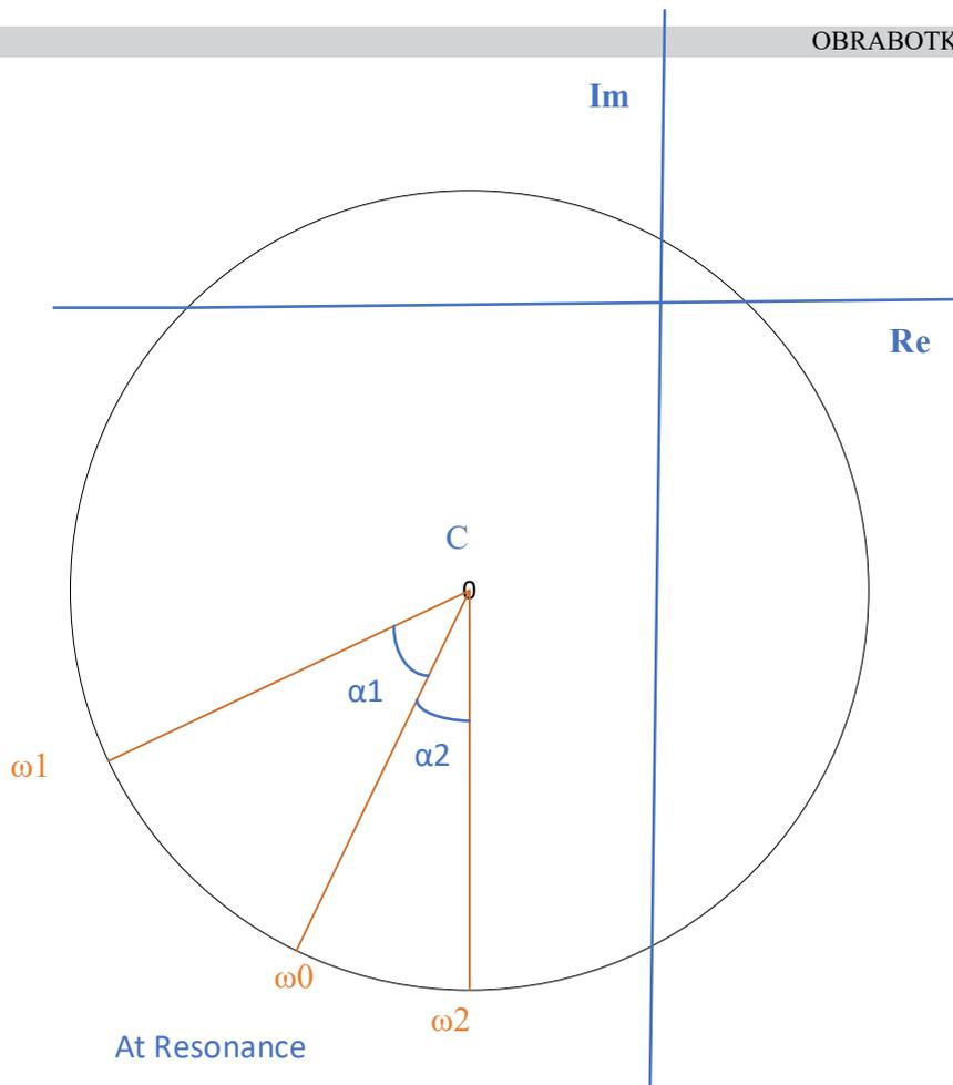
Fig. 5. Nyquist plot for fitting circle method
