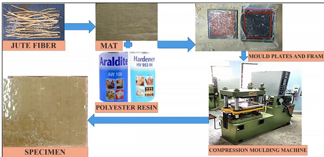
Fig. 2. Composite preparation flow diagram
