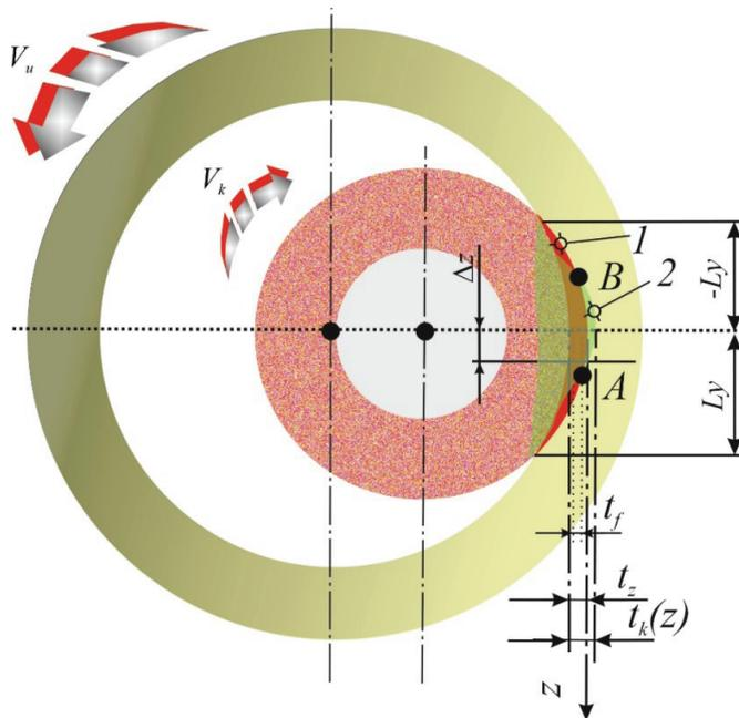
Fig. 1. Influence of vibrations on the depth of microcutting during internal grinding
