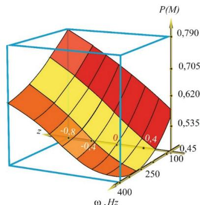
Fig. 3. Change in the probability of material removing along the contact zone from the level of grain penetration in the workpiece material during internal grinding at a relative vibration value of 100 Hz
