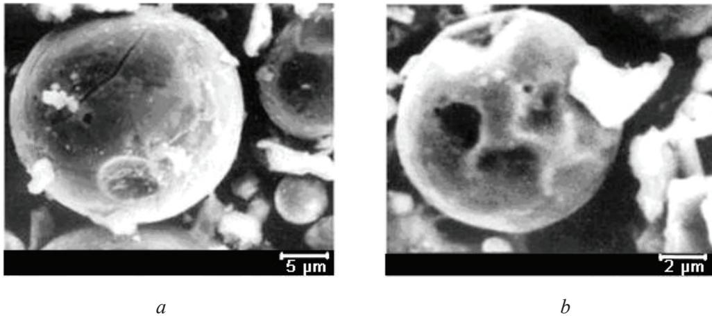
Fig. 2. The surface of spherical sludge particles after destruction:
