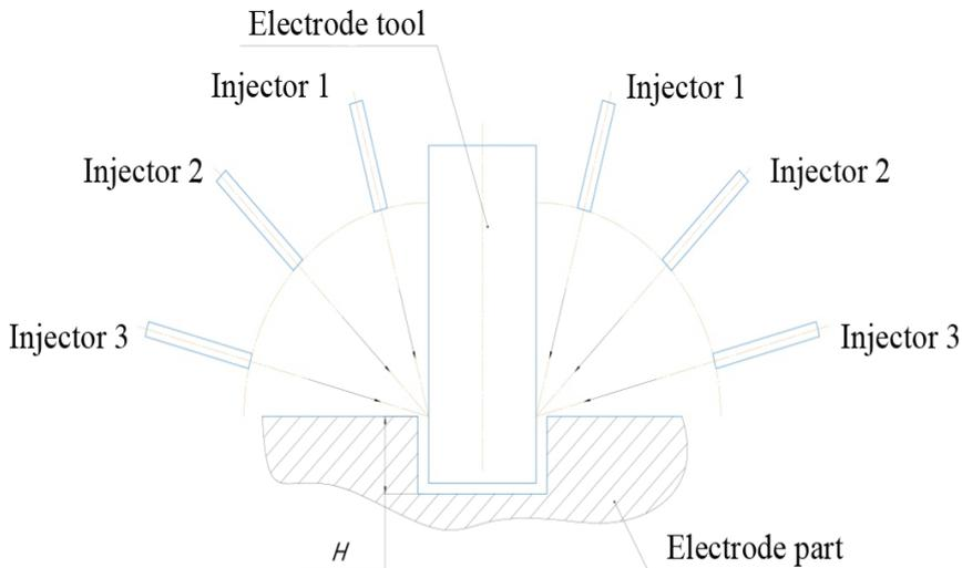
Fig. 5. Processing model, where  $H$  is the depth of processing
