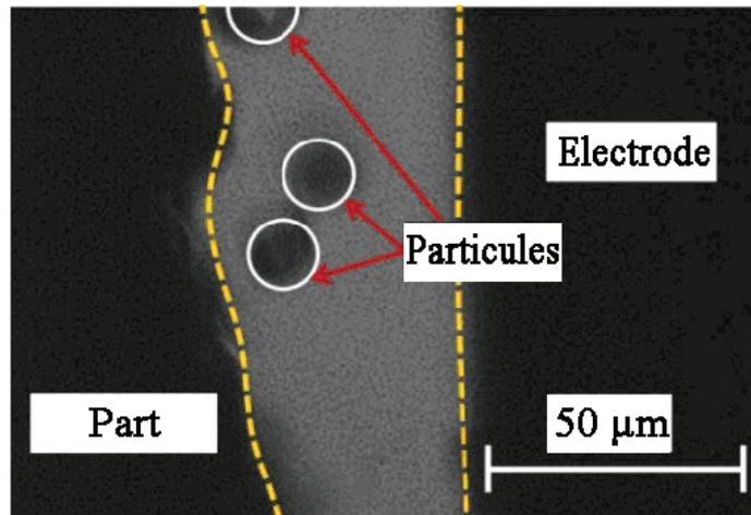
Fig. 3. Partial tracing in the gap between the electrode and the workpiece. The average particle velocity is approximately 0.75 m/s
