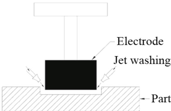
Fig. 4. Scheme of jet or side flushing
