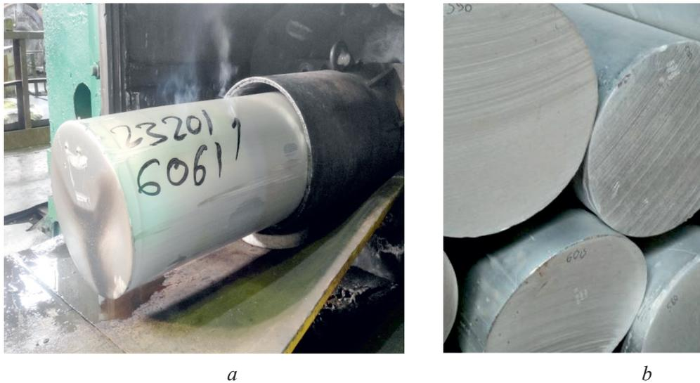
Fig. 2. The front of the rod at the exit of the die (a) and the cutting surface of the rods (b)
