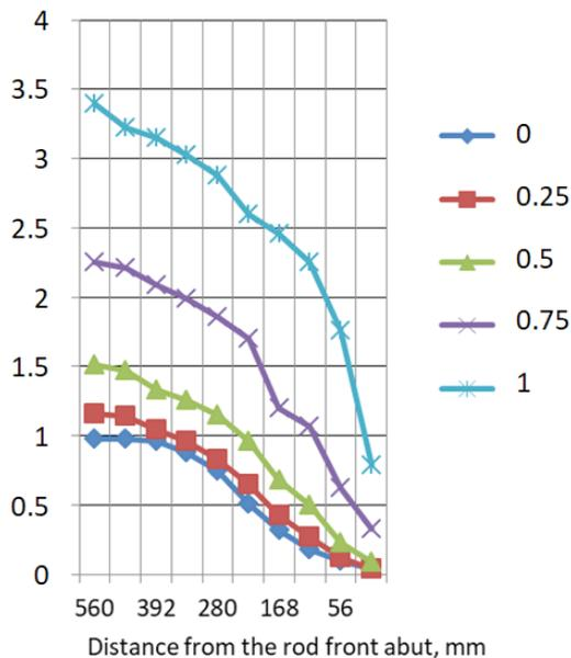
Fig. 5. Graph of the distribution of the strain degree in the cross sections of the rod depending on the distance from the front end at various relative radial coordinates  $r/R$
