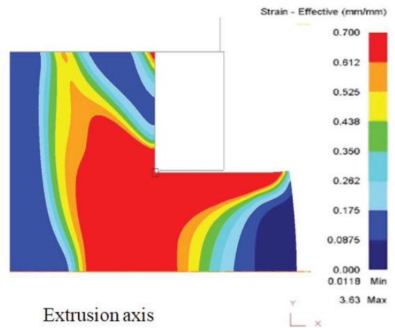
Fig. 4. Distribution of the strain degree in the longitudinal section in the nonstationary initial stage
