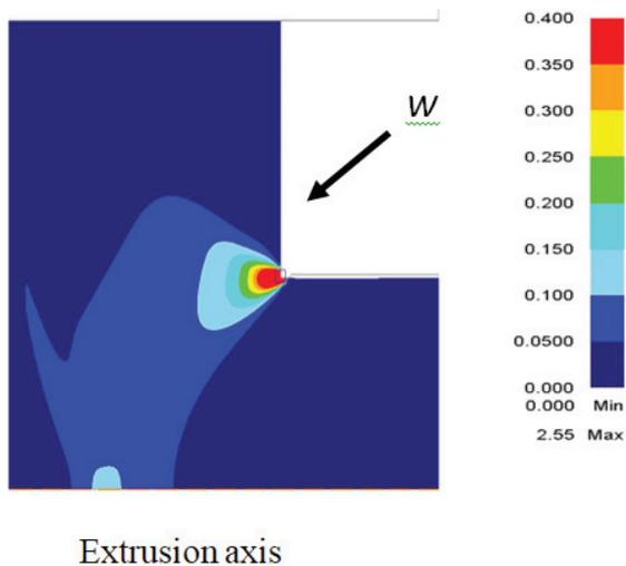
Fig. 6. Strain rate distribution (1/sec) in the longitudinal section (shape of the deformation zone);  $W$  – maximum point
