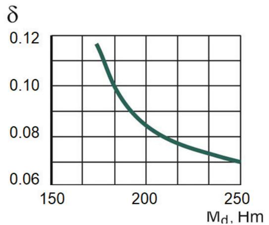
Fig. 6. A graph of the change in the value of the rotation irregularity depending on the value of the torque
