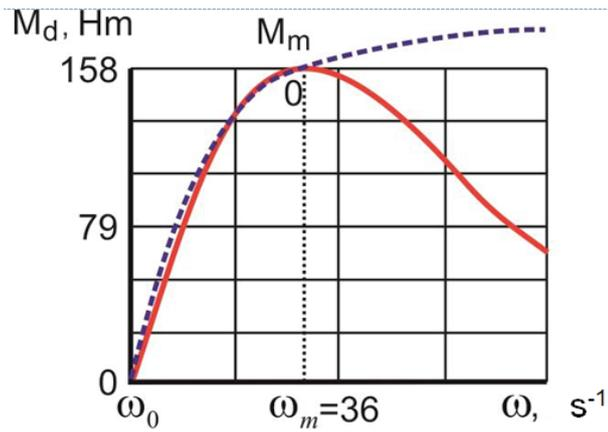
Fig. 2. Graph of an asynchronous motor and its special points
