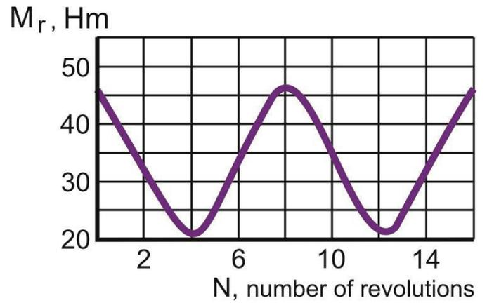
Fig. 3. The moment of resistance, reduced to the main (modified) shaft
