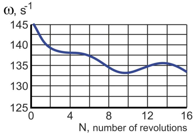
Fig. 4. Speed depending on the revolutions of the drive shaft
