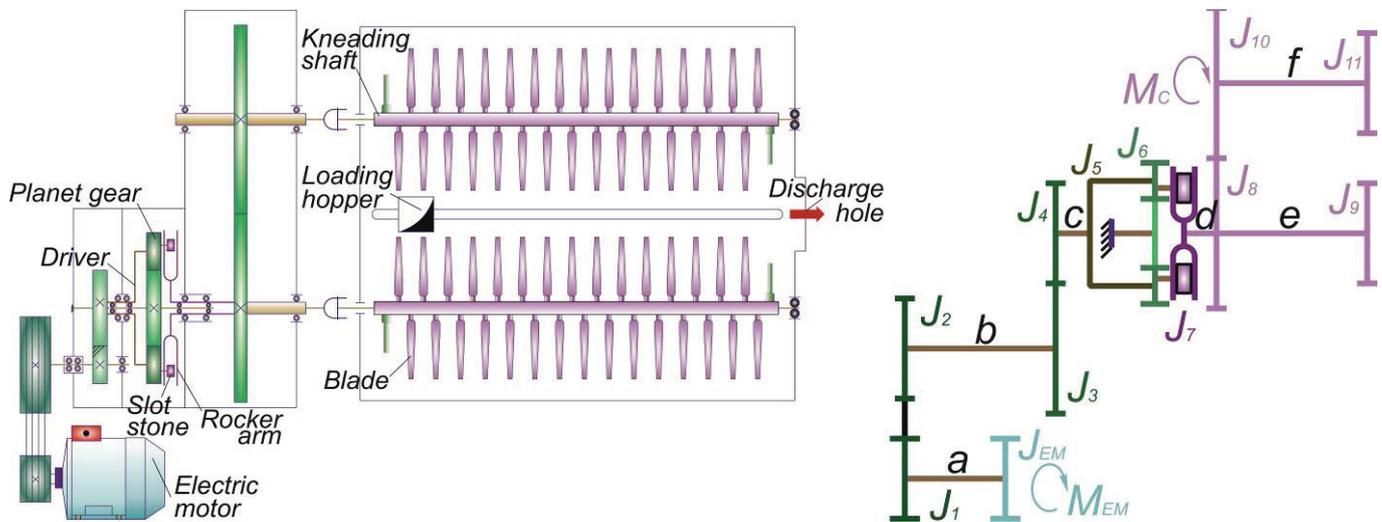
Fig. 1. Kinematic diagram and mathematical model of the kneader design that includes an epicyclic gearing
