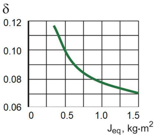
Fig. 5. A graph of the change in the value of the rotation irregularity depending on the mass moment of inertia
