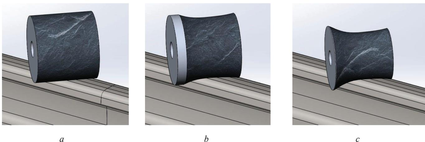
Fig. 4. The scheme of breaking-in of an abrasive wheel by HSG technology:
