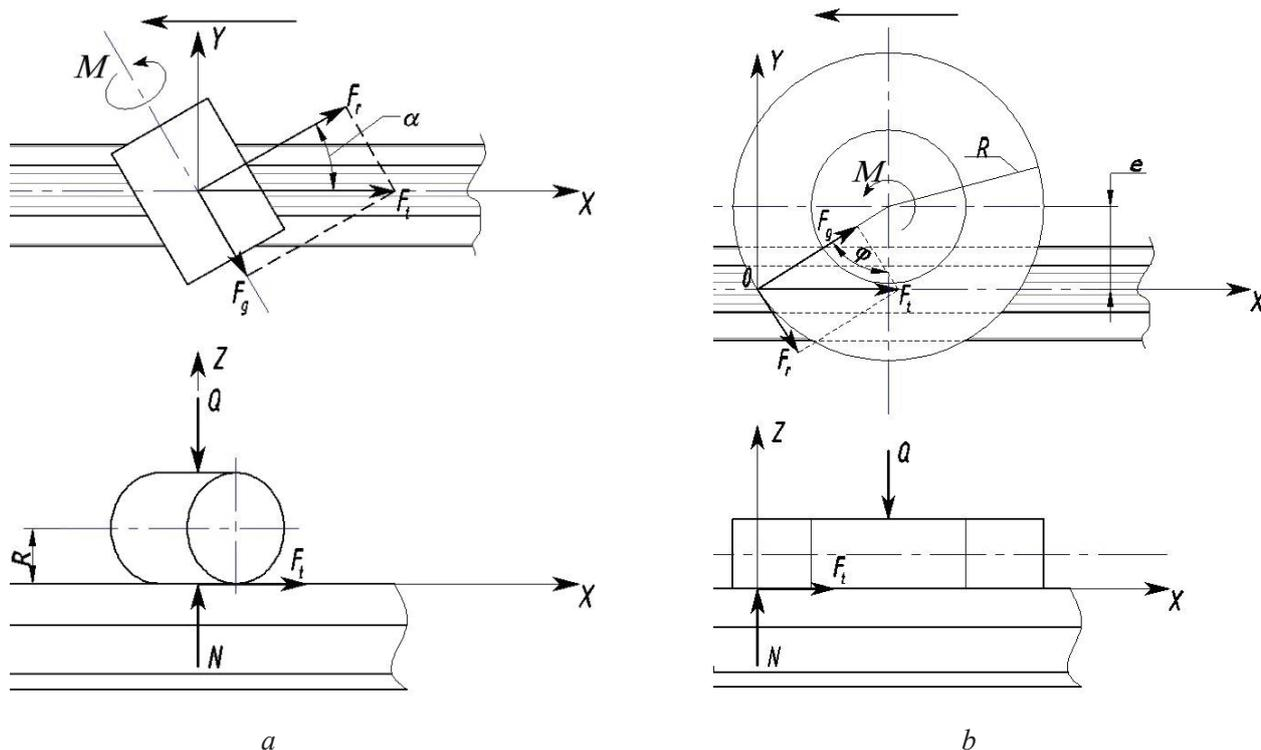
Fig. 9. Force interaction of grinding wheels schemes:
