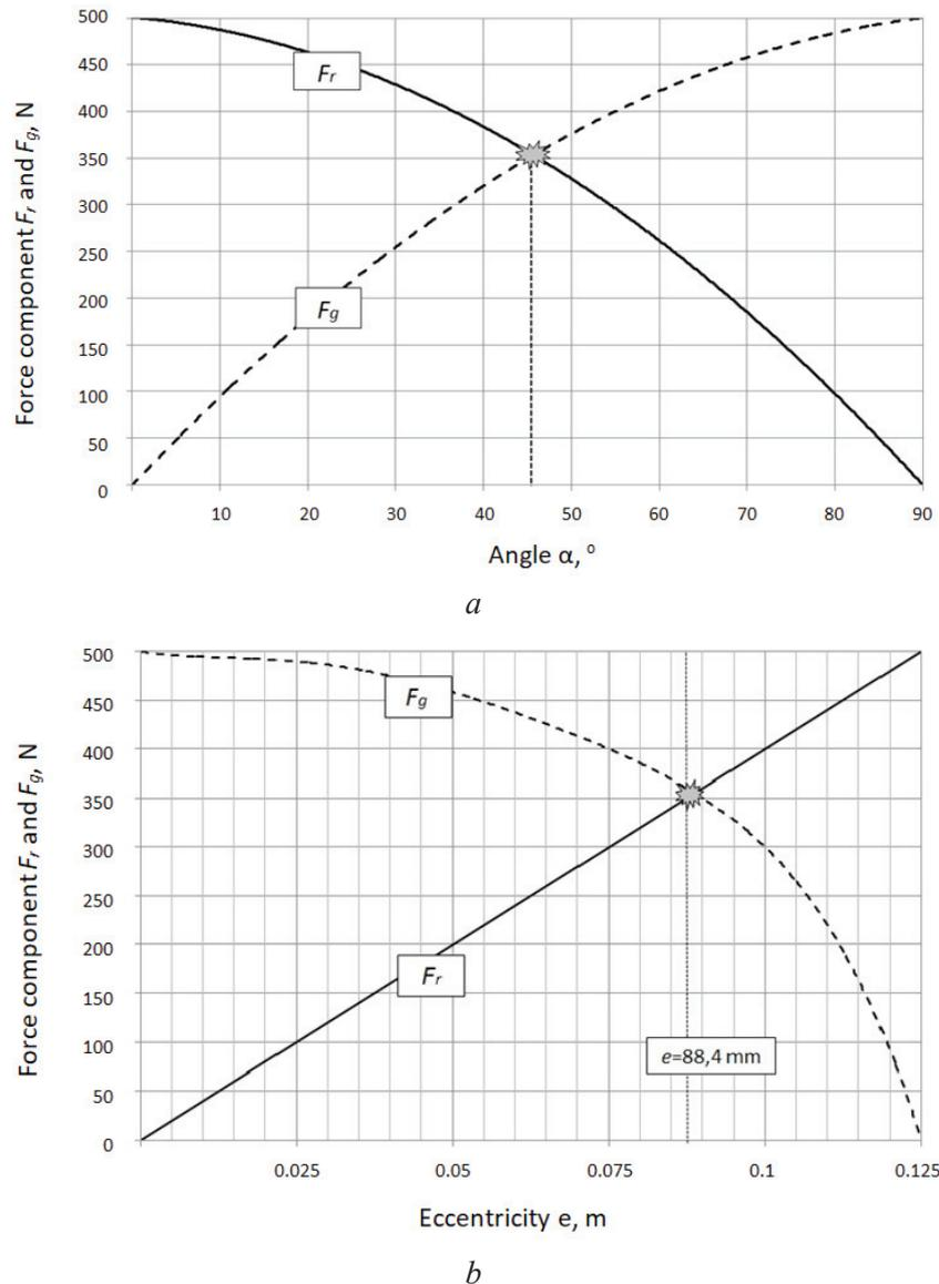
Fig. 10. Graphs of variance in components of force action on a grinding wheel at  $Q = 500$  N,  $\lambda = 1$  and  $R = 125$  mm:
