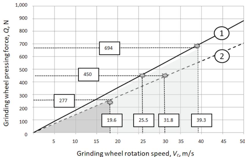
Fig. 11. The dependence of a grinding wheel rotation speed on the force of its pressing against rail at optimal values  $\alpha = 45^\circ$  and  $e = 88.4$  mm:
