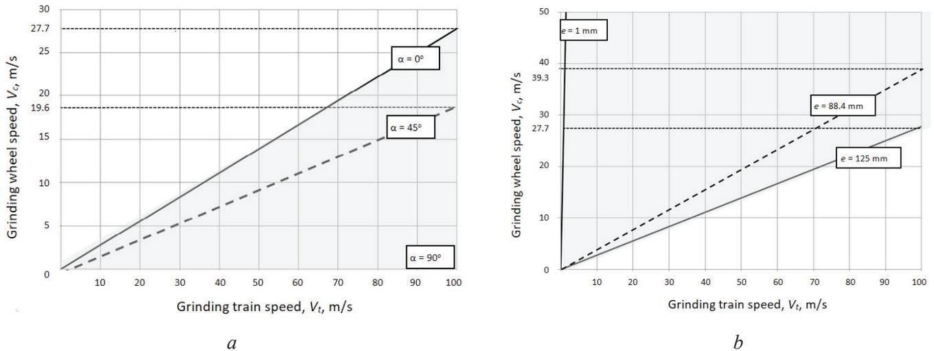
Fig. 8. Dependence of a grinding wheel rotation speed on grinding train speed:
