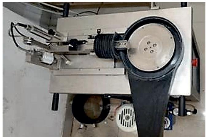
Fig. 1. A pin-on-disk machine showing disk arrangement
