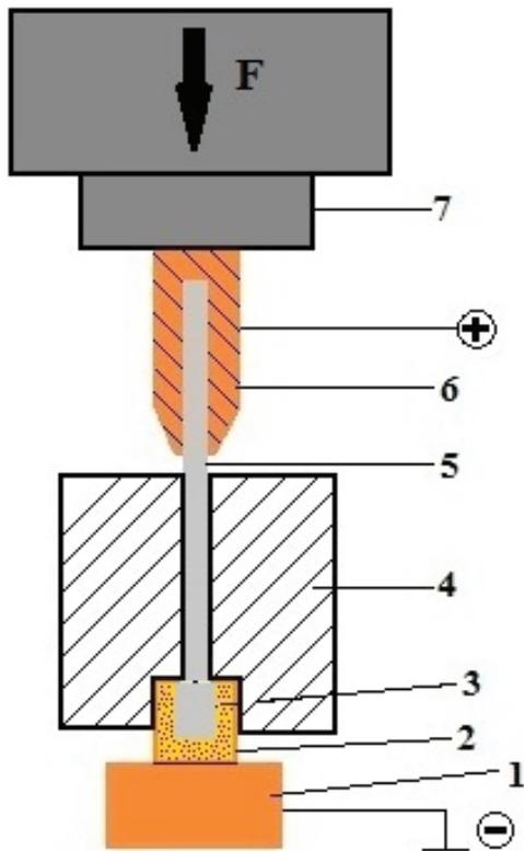
Fig. 1. Scheme of capacitor welding of a steel shank to the working part:
