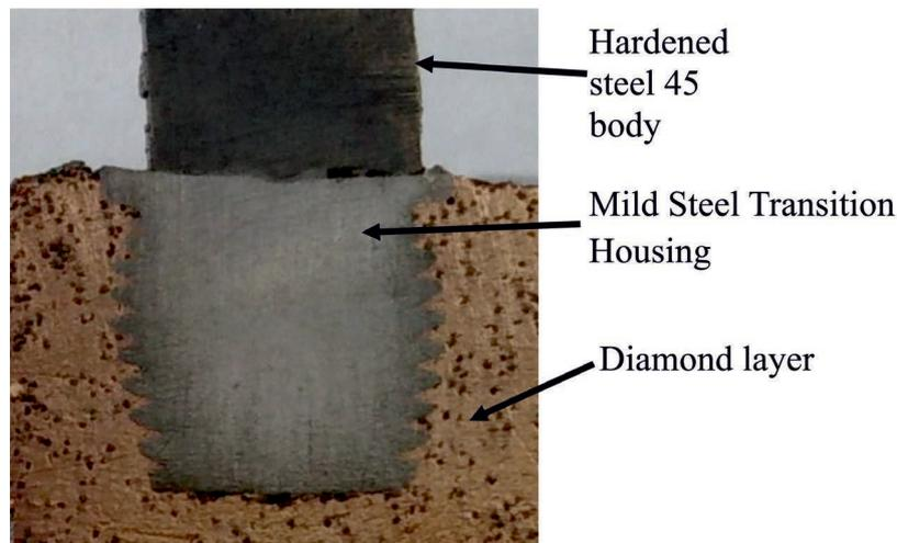
Fig. 3. The macrostructure of the welded joint area of the investigated diamond grinding head
