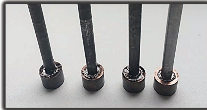
*Fig. 2.* Experimental samples of diamond heads with a diameter of 12 mm, made using the method of capacitor welding
