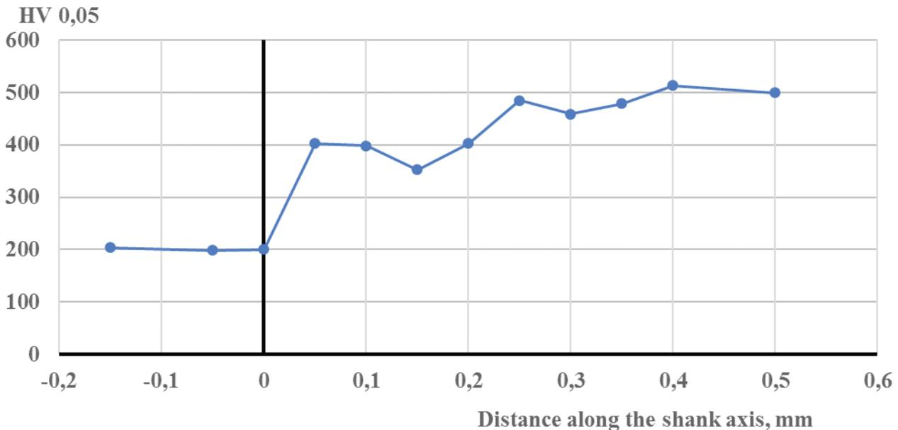
Fig. 4. Change in microhardness in the area of the welded joint of the body with the transition body of the diamond grinding head
