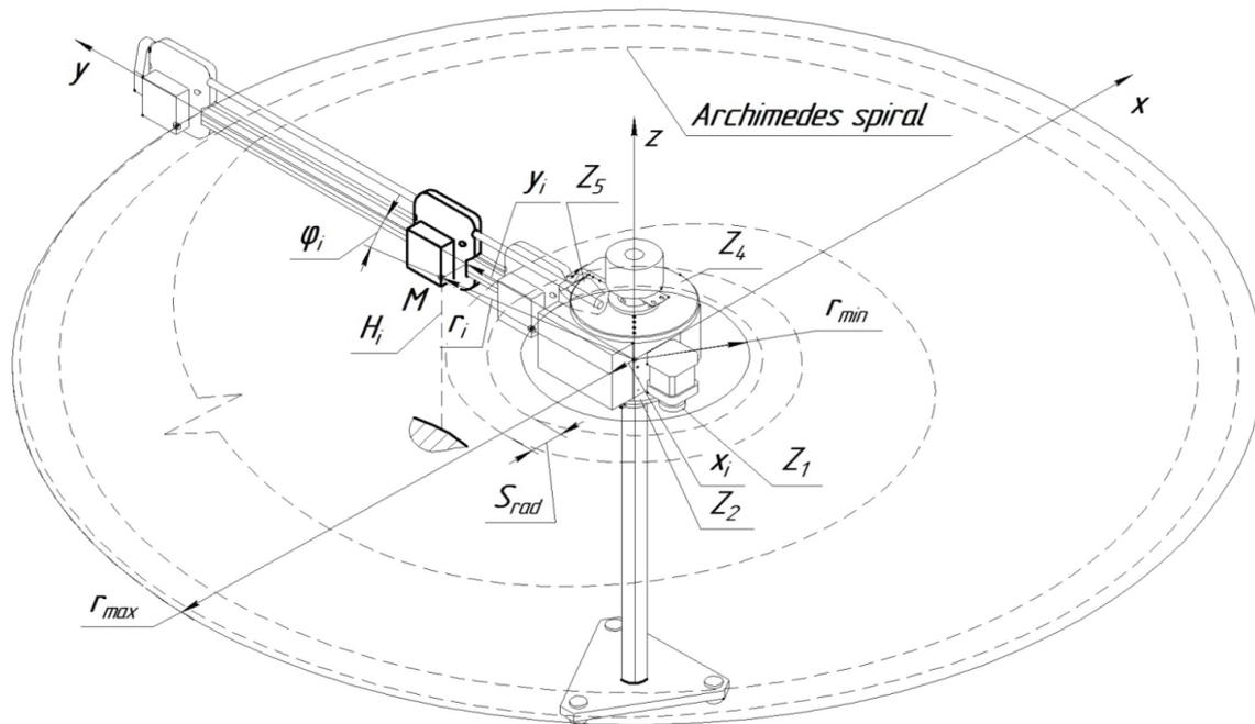
Fig. 2. The trajectory of the  $M$  point of the laser sensor
