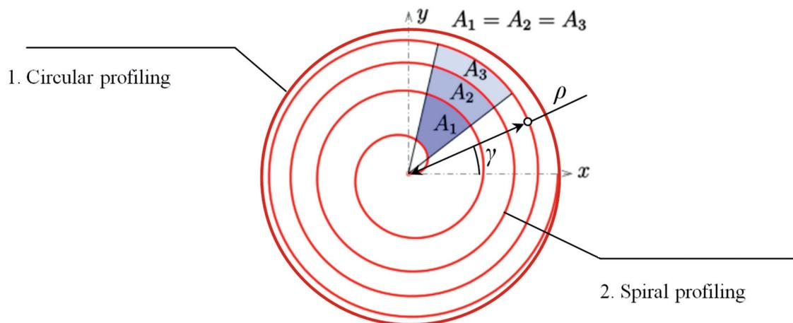
Fig. 4. Trajectory of the sensor movement in a circle and a spiral
