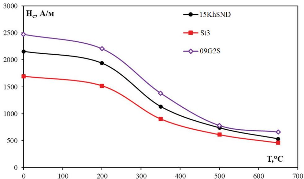
Fig. 7. Dependence of the coercive force on the tempering temperature of the investigated steels
