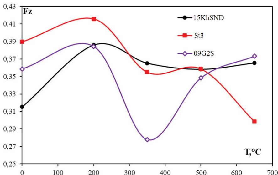
Fig. 4. Change in the value of the factor of different grain size  $F_z$  for samples made of 15KhSND steel with different heat treatment [20]
