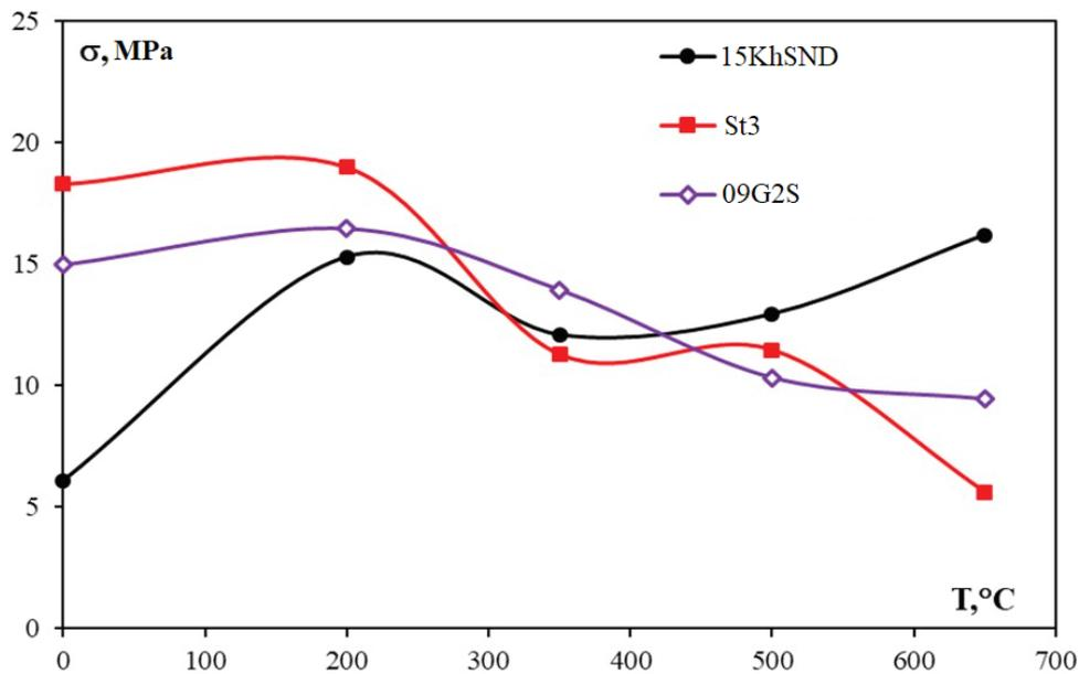
Fig. 5. Dependence of the change in the magnitude of internal stresses on the tempering temperature of structural steels
