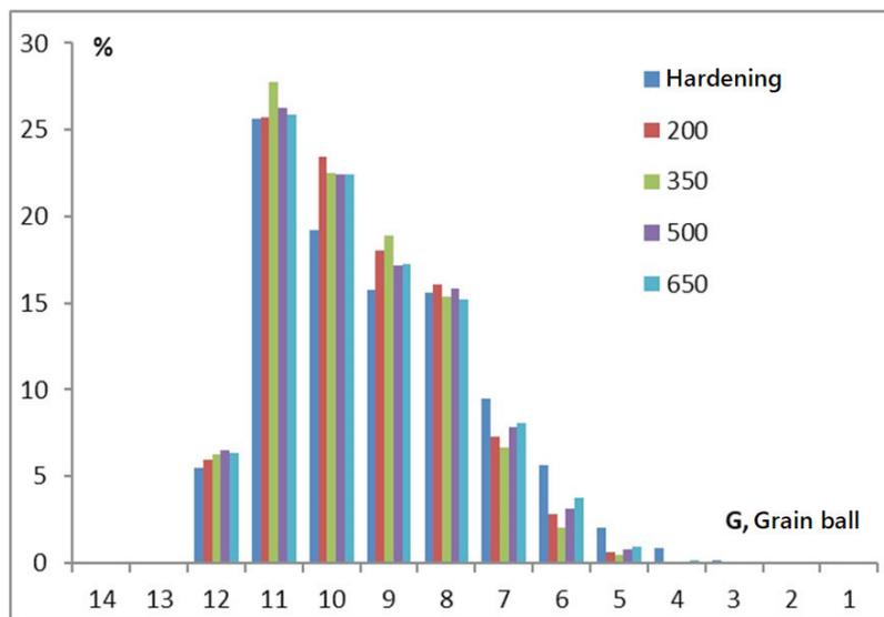
Fig. 3. Histogram of the percentage distribution of grains by points for micro-sections of heat-treated samples made of 15KhSND steel by grain size [20]
