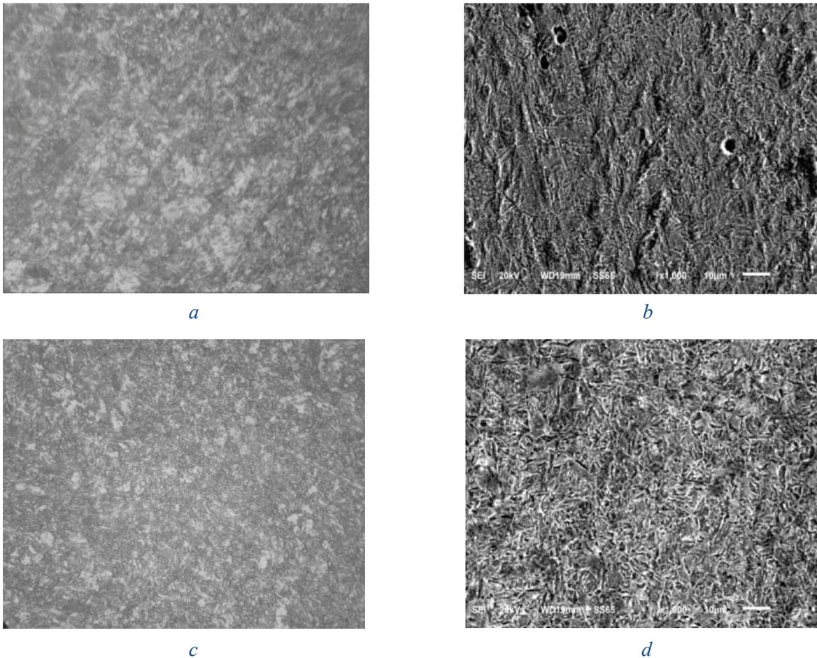
*Fig. 1.* Structure of heat-treated steel samples 09G2S at 1,000x magnification in optical and scanning electron microscopes:
