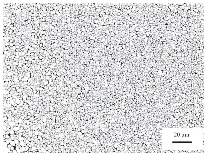
*Fig. 2.* Microstructure of a sample heated to 930 °C and quenched in water, made of rolled steel 09G2C, obtained by processing microphotographs in the SIAMS 700 software package
