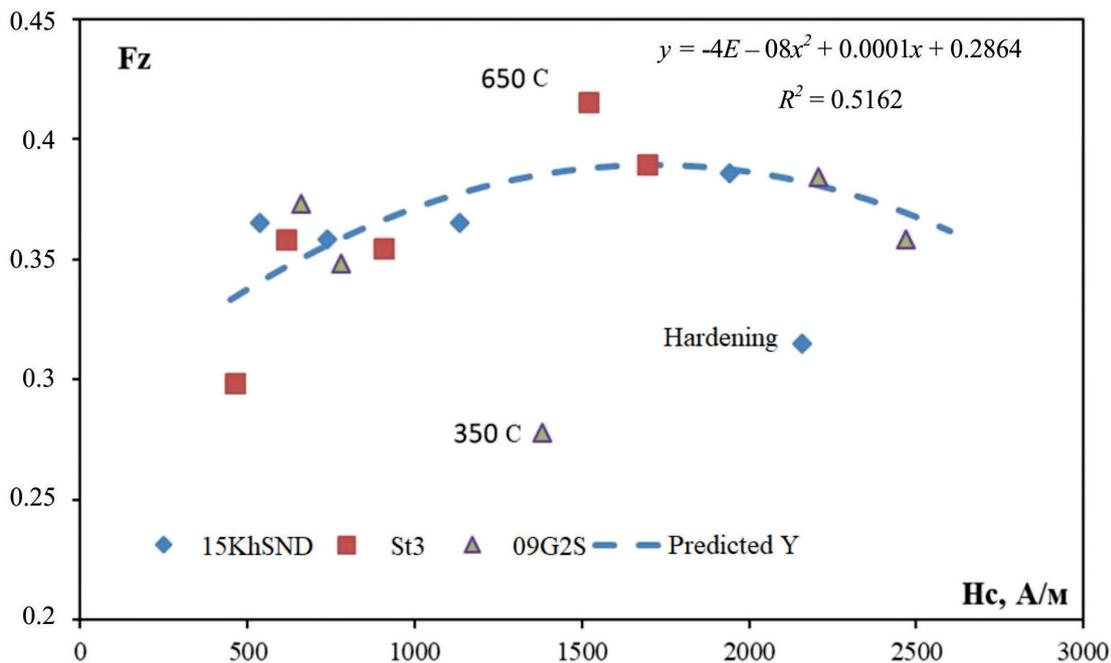
Fig. 10. The value of the factor of different grain size  $Fz$  depending on the value of the coercive force for heat-treated specimens made of structural steels
