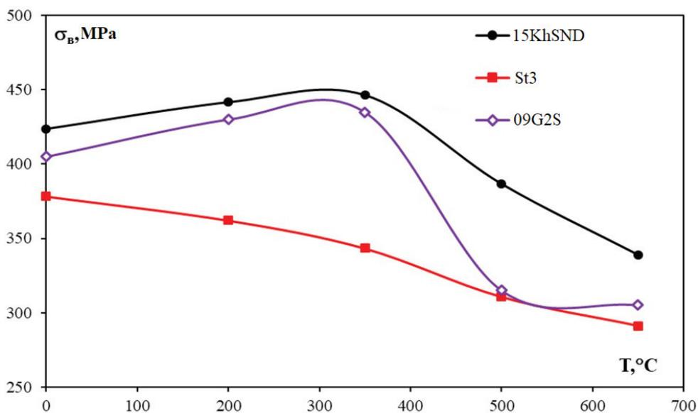
Fig. 6. Dependence of the change in the value of the ultimate strength on the tempering temperature of structural steels
