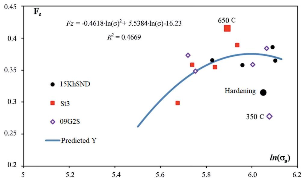
Fig. 9. The value of the factor of different grain size  $F_z$  depending on the logarithm of the ultimate strength value for heat-treated specimens made of structural steels
