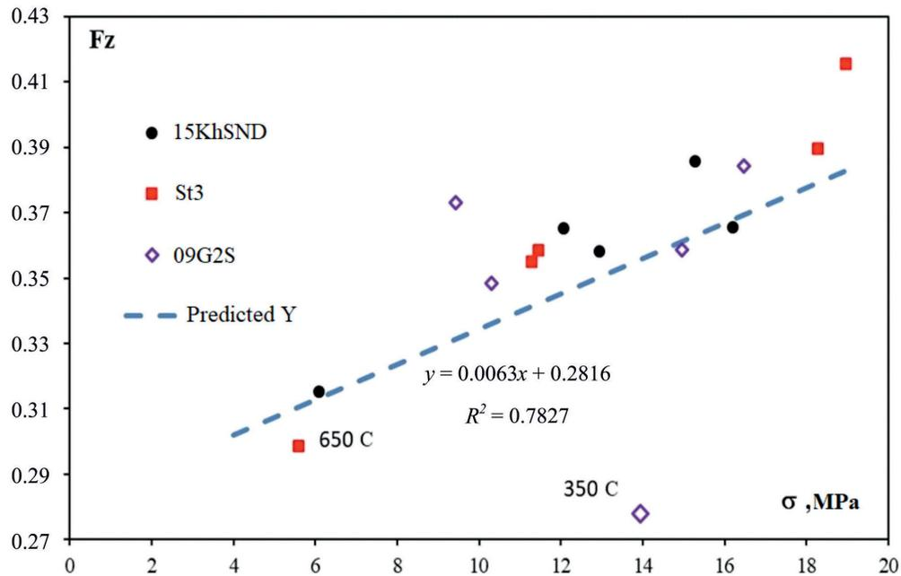
Fig. 8. The value of the grain size factor  $F_z$  depending on the value of internal stresses (stresses of the second kind) for heat-treated samples made of structural steels
