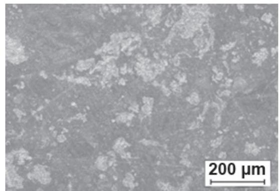
Fig. 5 SEM image of the surface of a sample of ceramic  $\text{B}_4\text{C-TiB}_2$
