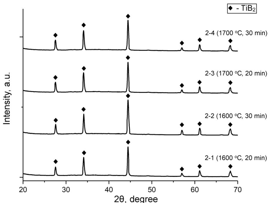
Fig. 3. Diffraction patterns of titanium diboride samples
