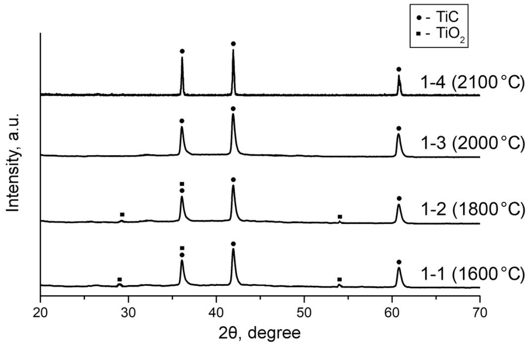
Fig. 1. Diffraction patterns of titanium carbide samples
