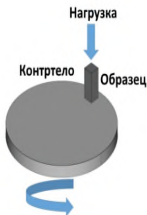
Fig. 2. Tribological loading scheme “pin-on-disc”
