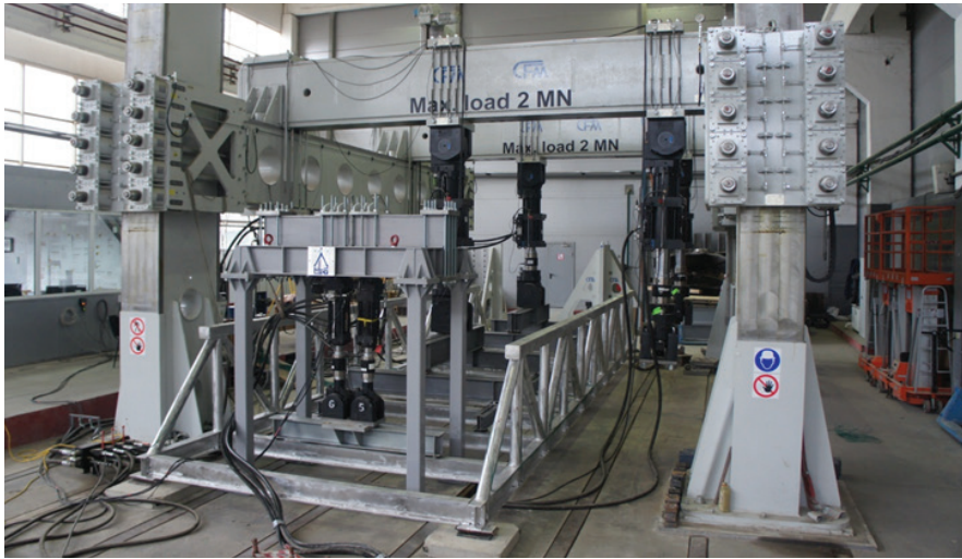
Fig. 11. Endurance tests of the load-bearing frame of a pedestrian bridge on the test bench of the Moscow State University of Civil Engineering and Architecture (NRU MGSU)
