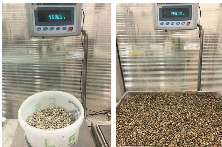
Fig. 4. Determination of dust and clay particles content in dolomite aggregate
