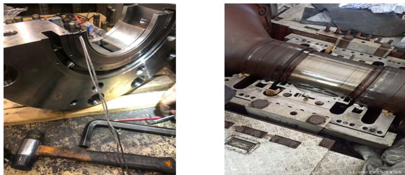
Figure 2. Bearing damage due to the misalignment in a gas turbine of the Kirkuk power plant located in Iraq
