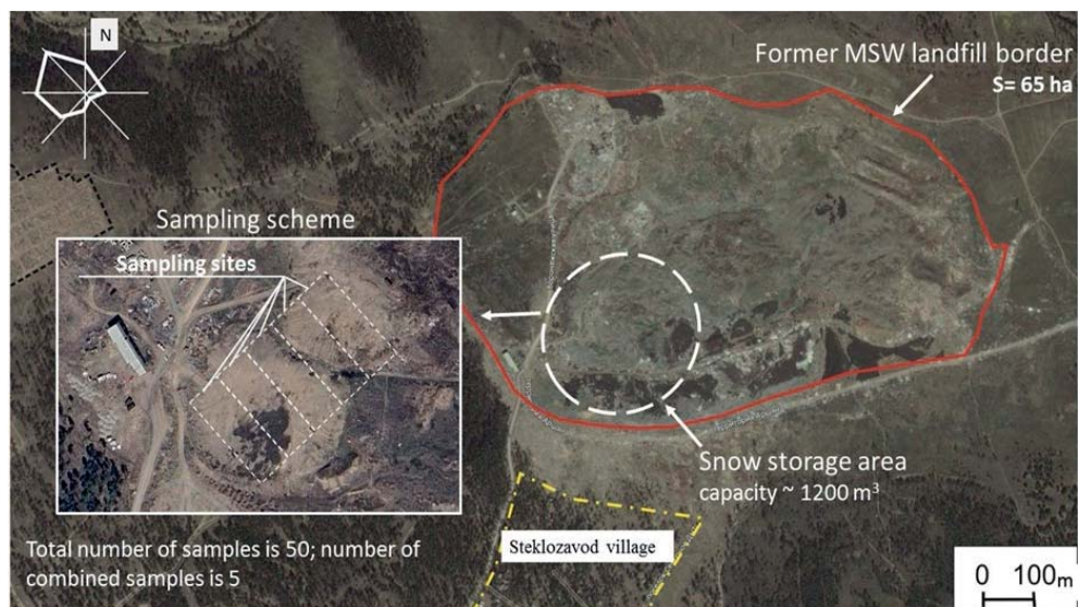
Figure 1. Sampling scheme at the snow accumulation site Source: compiled by T.V. Cheredova, O.N. Chudinova.
