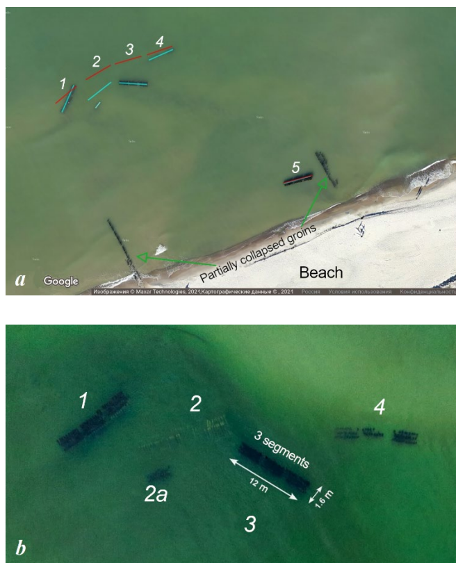
Fig. 3. Initial and final location of the “Grebenska” breakwater modules: a – initial (red lines) and final (blue lines) location of the modules (Google Maps image, 2021. https://www.google.ru/maps ); b – location of the “Grebenska” breakwater modules on 12 April 2023
