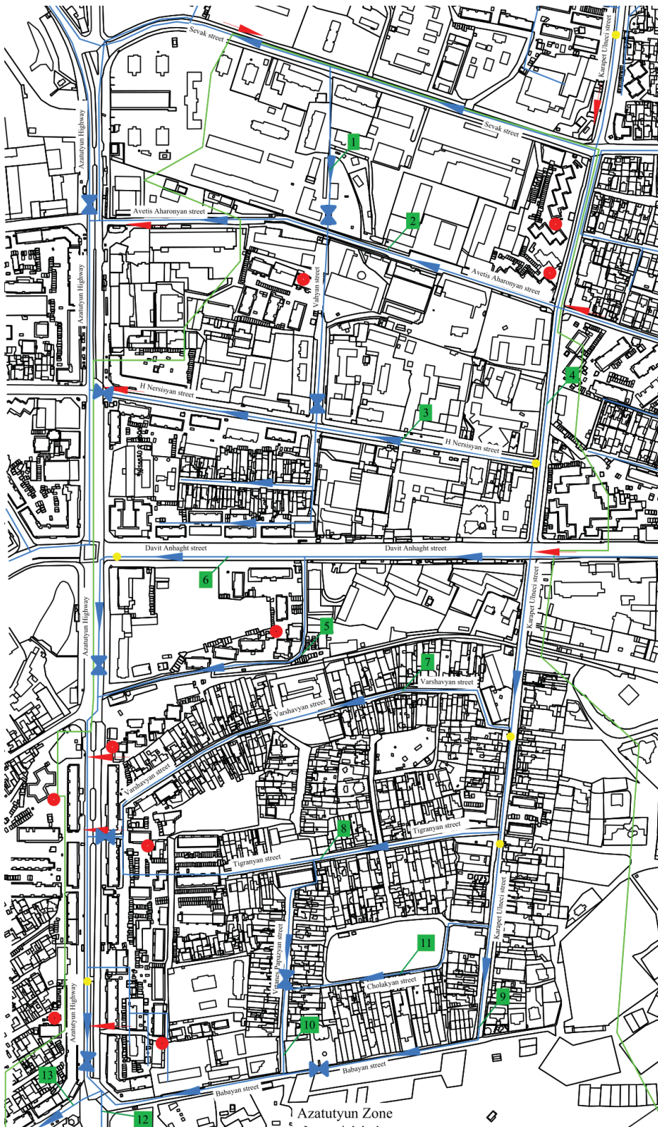
Fig. 2. Scheme of water supply zone in Inner Zeytun district: → – eliminated hydraulic connection; → – water flow direction; ● – pump station; ● – PRV; ↔ – closed valve; — – zone initial boundary; — – pipelines
