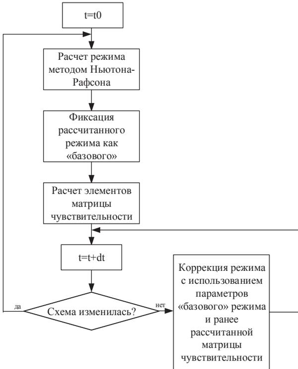
**Fig. 1.** Block diagram of the algorithm for determining the operating mode parameters of the distribution electrical network
