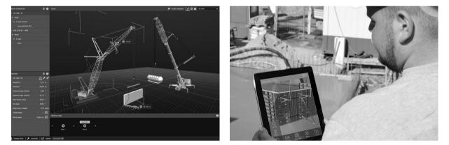
Fig. 7. Crane Planner software and the planitec AR app
