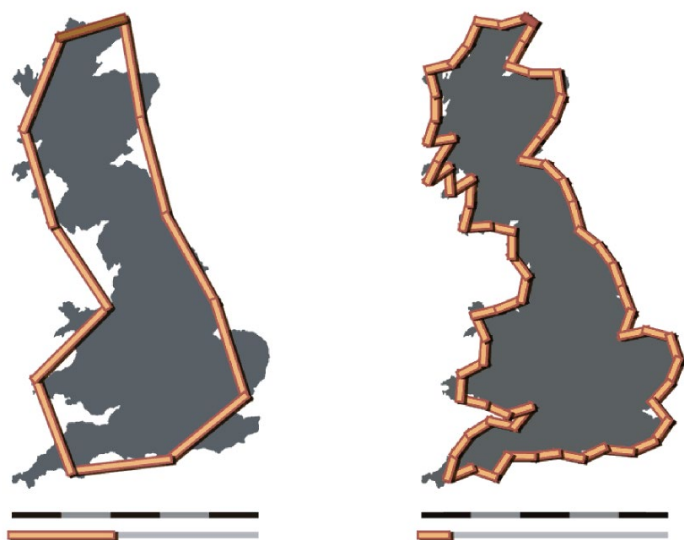
Fig. 1. The coast of the Britain measured on several scales left: Unit = 200 km, length = 2400 km (approx.) right: Unit = 50 km, length = 3400 km Reprinted from Wikipedia project page
