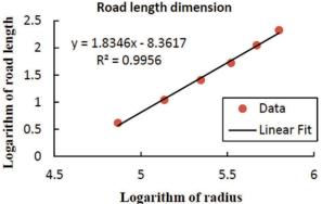
**Fig. 2.** Detection of fractal structure for the road network in Strasbourg, France. Adopted from (Wang et al., 2017)
