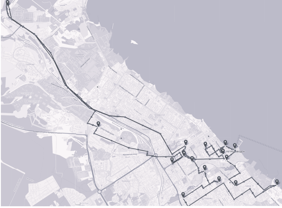
Figure 4. Solutions for the TSP on the Petrozavodsk dataset (18 POIs) by the QA approach with n_q = 12 , tour length 47488 steps
